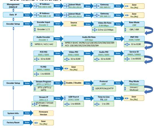
All commands and settings are also available on Web based configuration by connecting the Ethernet port of computers to the NMS port of MP-200. Launch any Web browser and point the URL to http://192.168.0.168 to login with
